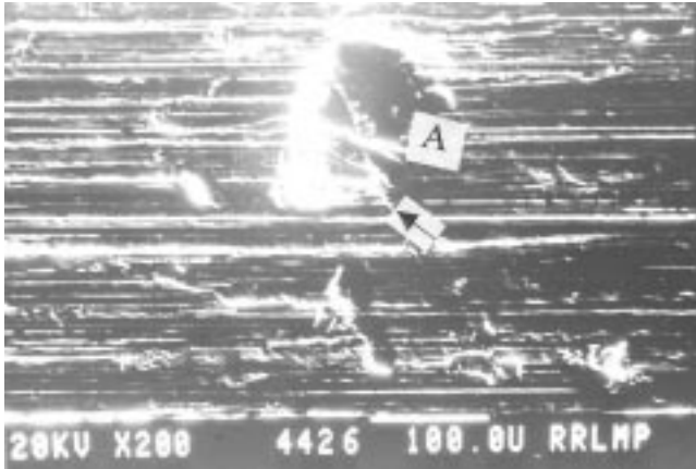
Fig. 9 Wear surface of mild steel
